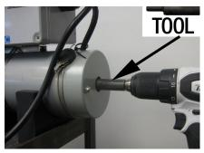
In Case of a Power Outage This Tool May be Inserted Into a Drill to Raise or Lower Your Lift. First Remove Rubber Cap From the Motor Shaft.
