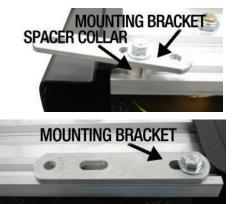
3. This Lift has Two Options. One for Left or Right Mounting. Install the Mounting Bracket.
