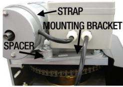
6. Install the Strap Around the Motor and Connect the Strap and Mounting Bracket with the Spacer Provided. Pictures Above Show the Two Different Mounting Options Depending on What you Need.
